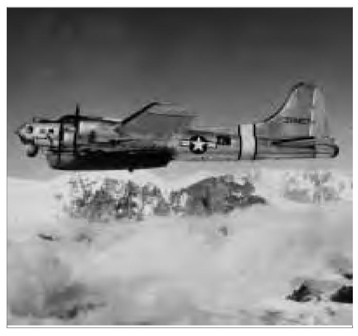
Although they were built to bomb, a few Boeing B-17s were converted for use as air rescue airplanes and, from their former bomb bay locations, dropped lifeboats in situations where a water landing wasn't possible. The lifeboats—like this one attached to a 10th Rescue Squadron SB-17 flying over Alaska—were suspended on three parachutes. They were self-righting and came with self-bailing equipment
